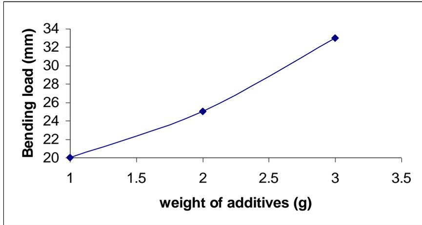
Fig(6) Effect of Resorcinol additives on bending load of U.M.F
