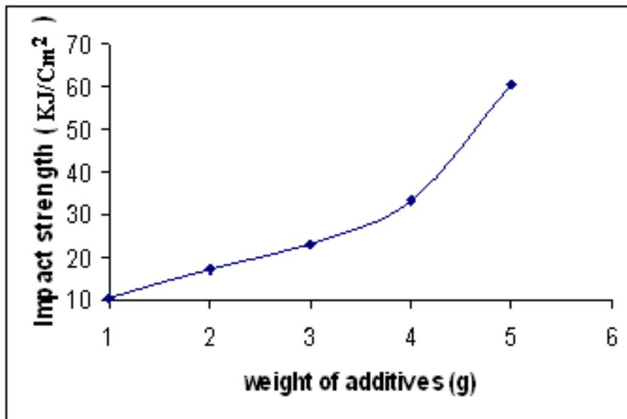
Fig(1) Effect of urea additives on Impact strength of M.F
