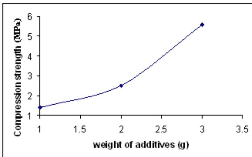
Fig(5) Effect of Resorcinol additives on compression strength of U.M.F
