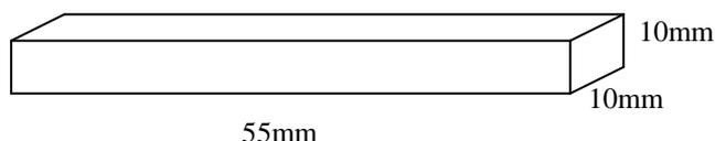
Fig. (1) Dimensions of sample used in impact test.
