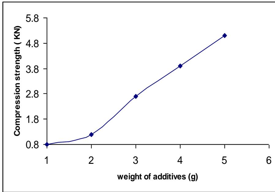
Fig(2) Effect of urea additives on compression strength of M.F
