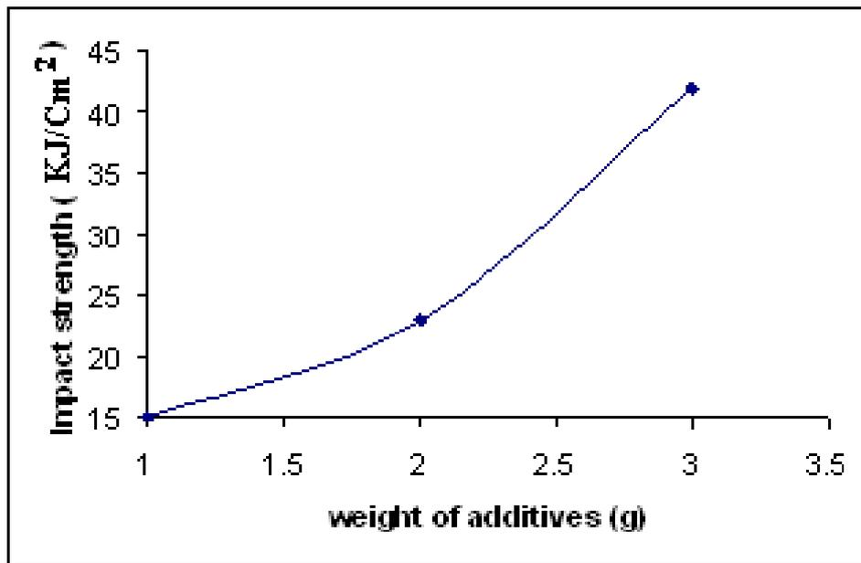
Fig(4) Effect of Resorcinol additives on impact strength of U.M.F
