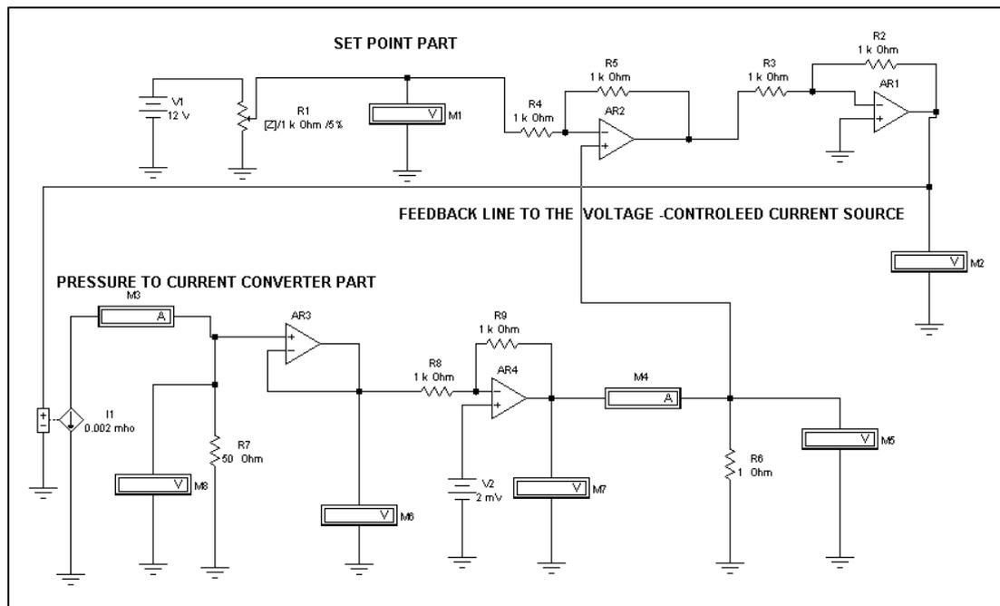
Figure (9) the designed proportional controller card.
