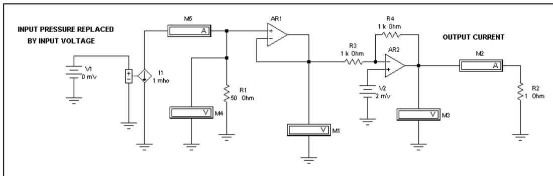
Figure (5) simulation of the pressure transmitter.
