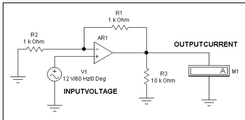
Figure (3) voltage to current converter.
