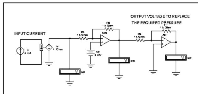
Figure (8) simulation of the current to pressure converter.
