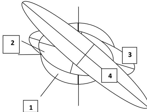
Fig (5) calculated field dependence of the laser polarization in multimode when 1:H=0 Gauss, 2:H=2 Gauss , 3:H=5 Gauss, 4:H=6 Gauss.
