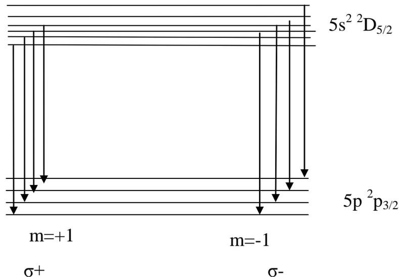
Fig(1)energy levels of the He-Cd 4416Å Laser transition in magnetic field
