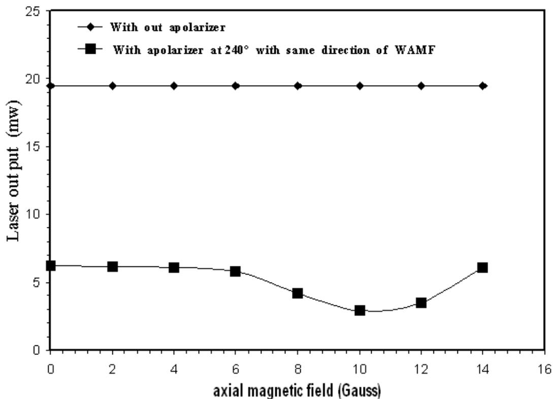
Fig.(6b).laser output as a function of the WAMF strength,(■) with a polarizer at 240° with same direction of WAMF, (◆) with out polarized . Table(2) laser output as a function of the WAMF strength with a polarizer at 150° , 240°with same direction of WAMF ,and 240° with reversed direction of WAMF,and also without polarizer.
