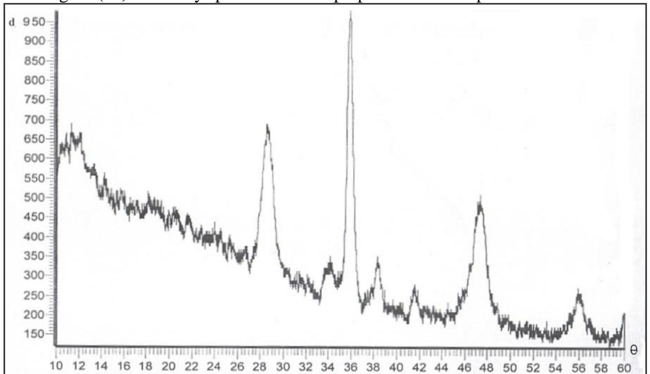
Figure ( 7 ) the X-ray spectrum of SiC prepare at 700 mJ/pulse
