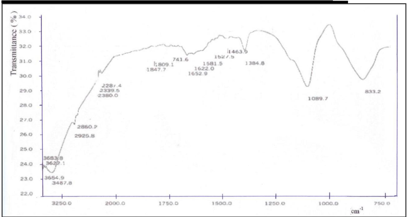
Figure ( 2 ) the FT-IR Spectrum of SiC prepared at 1 J/pulse
